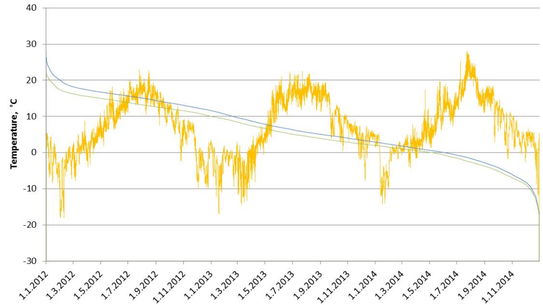
Ambient air: dry temperature and duration of dry and wet bulb temperatures Air data: hourly averages, Hanko/Tulliniemi 2012-2014 by FMI
